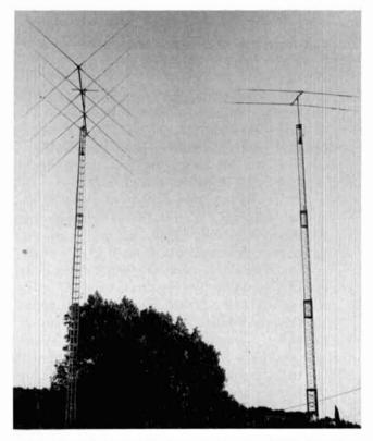
The enigmatic quad. This 4-element quad at K6NA, because of its mediocre performance, inspired Landskov's efforts to develop a competitive long quad. Now modified to Landskov's dimensions, it remains so marginal that the reference 2-element tribander nearly topped its gain midway across 15 meters. Were the reference beam a 3-element trap tribander, it would have probably matched or beaten this quad across all three bands.
